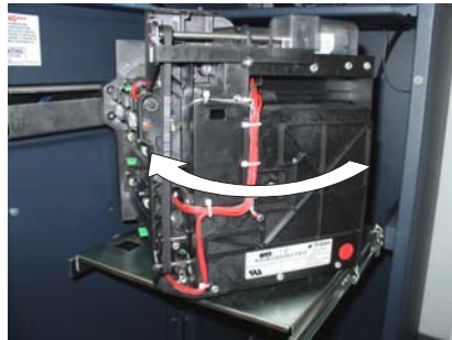
Rotate mechanism to “Service” position (clockwise).
