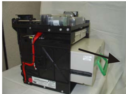
Removing note cassette (TDM-100).
