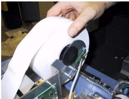
Figure 5-4. Place paper roll on bracket. Paper feeds from top of roll!
