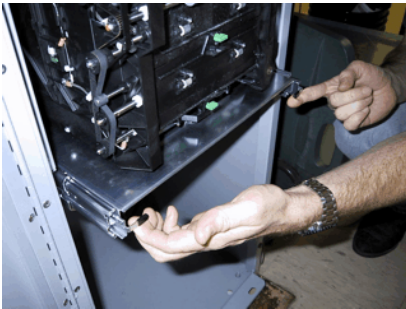
Lift up on slide tray locking levers.
