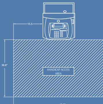
*The dimensions shown comply with US Federal ADA guidelines. For installation within the US, be sure to check state and local guidelines for complete compliance. For non-USA installations, check regulations for the country in which the machine will be installed.*
