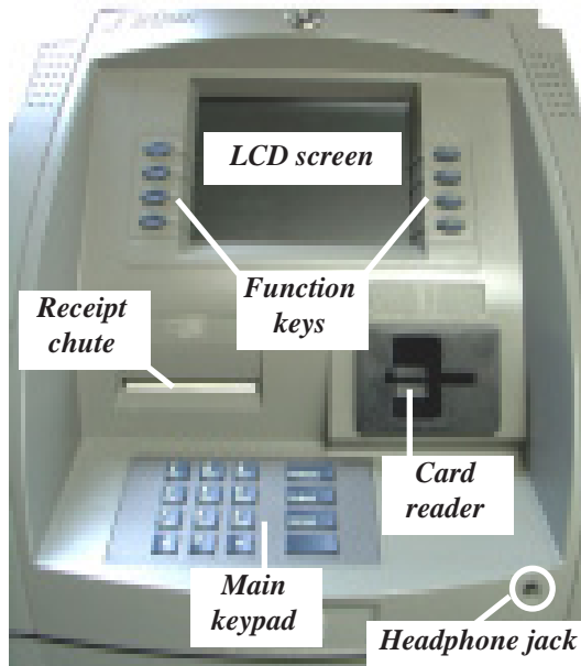
Figure 2-1. Control panel layout.
