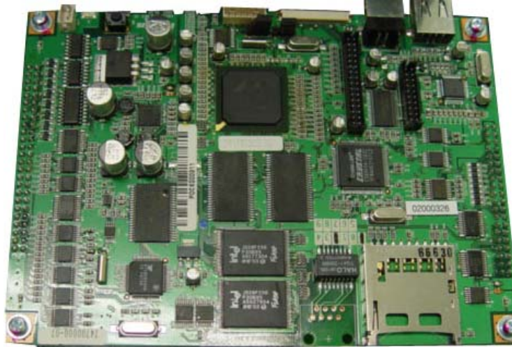
Fig. 3.8 Main Control Board
