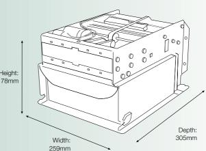
Mechanism without tray and notes: 5.3 kg Note Tray with inclusive reject compartment (without notes): 1.6 kg
