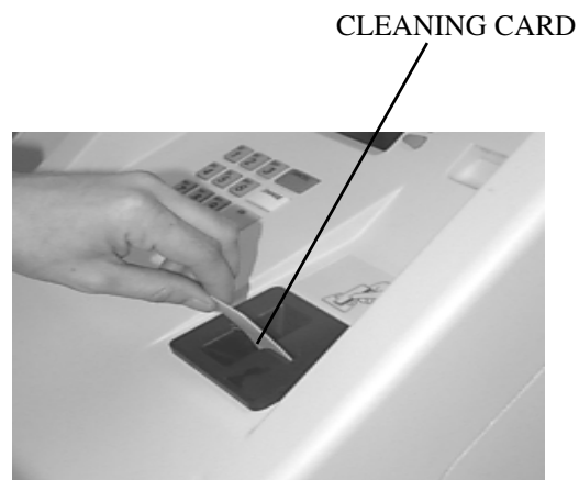
Figure 6-1. Use the cleaning cards on a monthly basis to maintain effective card reader operation.
