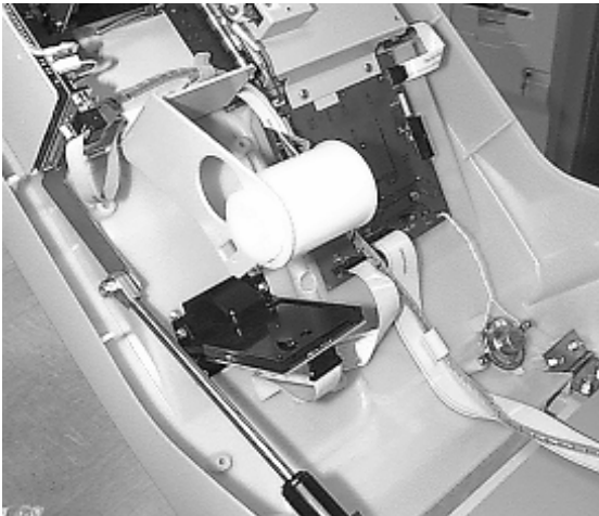
Figure 6-4A. Paper Spool in its normal operating position.
