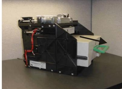
*Figure 4-6b. Removing note cassette. (TDM-150)*
