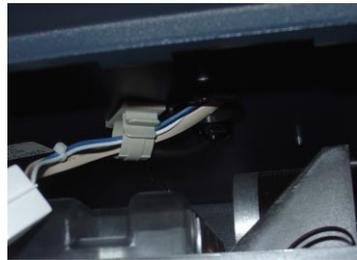
Figure 12. Cables routed through cable clip.
