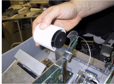
Figure 6-3. Removing paper roll from bracket.
